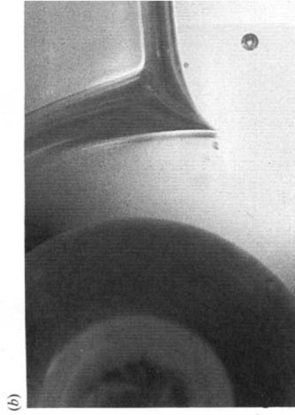
FIGURE 9. Critical speed for cusping of M1 in air is approximately 2.4 r.p.m., (a) 2 r.p.m., (b) 75 r.p.m. (cf. figure 6).
